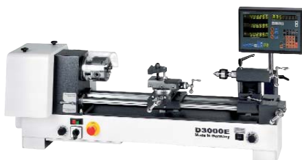
Illustration D3000 E with 3-axis digital readout system
