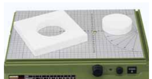
Crosscuts are achieved by means of a simple yet efficient solution: secure drawing-pin to table by means of a tape, it serves as a fixed centre.
