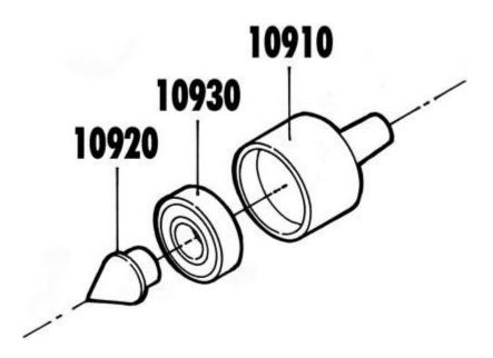
Note: The bearing and nose piece are pressed in at the factory. Once assembled, the 1191 Live Center is not considered user-serviceable. Parts are shown for reference only.
