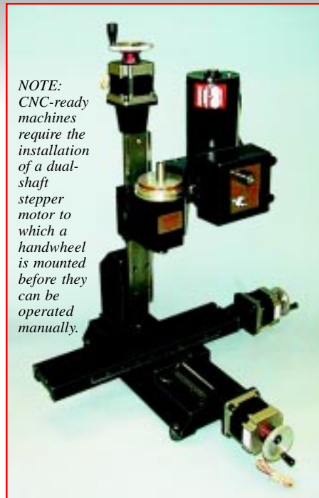
FIGURE 107 —Sherline offers CNC-ready mills with stepper motor mounts factory installed. Just add your own 23 frame size stepper motors and computer hardware/software or buy a turnkey setup from one of our CNC dealers.
