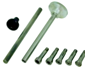
FIGURE 21—The WW collet set includes adapter, drawbar, knockout bar and five collets.
