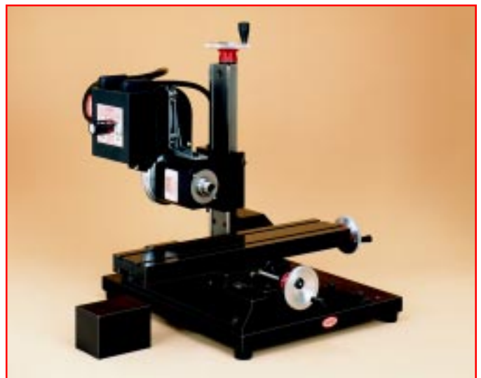
FIGURE 95—The horizontal milling conversion allows the column of the vertical milling machine to be repositioned in various ways on a specially machined base in order to provide greater versatility in set-up and increase the machinable area of the parts being worked on. Position "A" shown above takes advantage of the long 9" side-to-side X-axis travel. Another position 2-1/4" further from the table is useful for drilling operations. Shown to the left of the milling conversion baseplate is the base of the Z-axis column, which has been cut off to allow a lower positioning of the headstock in relation to the table.
