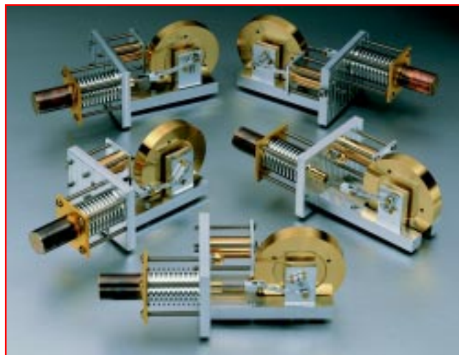
Project: Five identical Stirling hot air engines. Tim built this as his first project and made five of each part to improve his machining skills faster.
