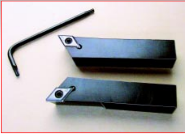
FIGURE 19—35° carbide insert holders and Torx wrench. The 3/8" shank fits in tool post P/N 7600.
