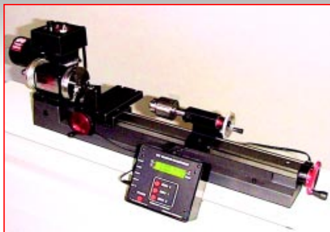
FIGURE 55—The digital readout indicates table position to within .0005" (.01mm) and also reads out spindle RPM.
