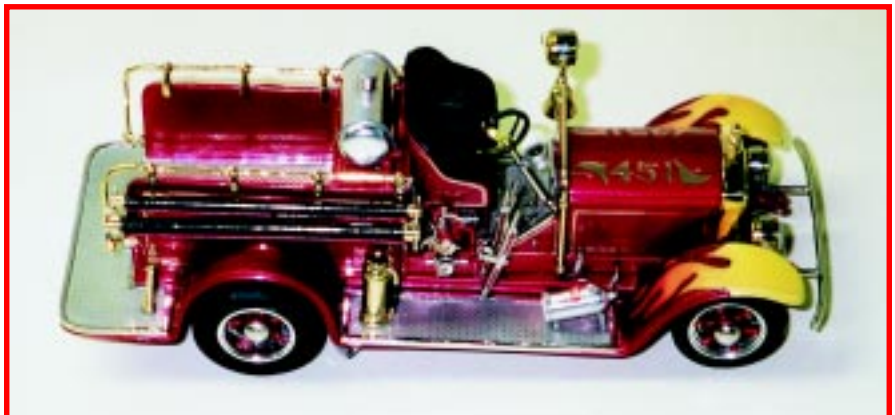
1/32 American LaFrance hotrod fire truck • Mike Foti, Hillsboro, OR Mike's entry in the hotrod division of the 1999 Salt Lake City national model contest is made entirely from formed and soldered brass. Items like the wheels, gas tank, lights, bell and rail stanchions are turned on the lathe.
