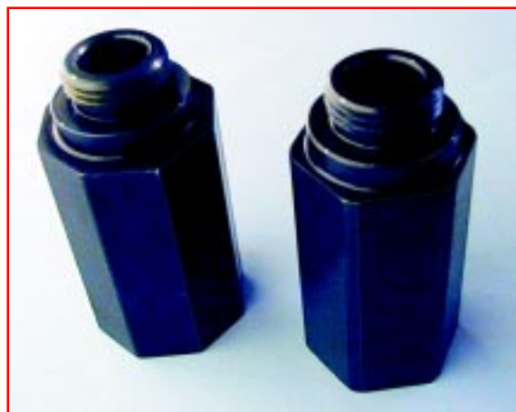
FIGURE 82 —An indexing set offers an easy way to index simple hole patterns or do milling on 2, 3, 4, 6 or 8 sides.
