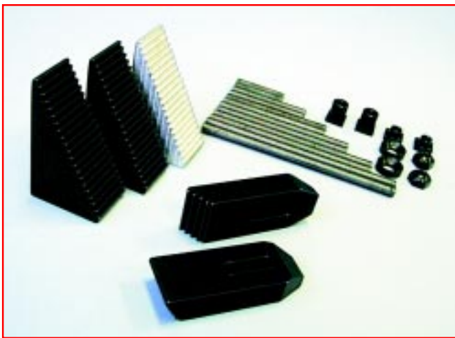
Figure 77—A step block set offers a quick and versatile way to clamp parts to the mill table.
