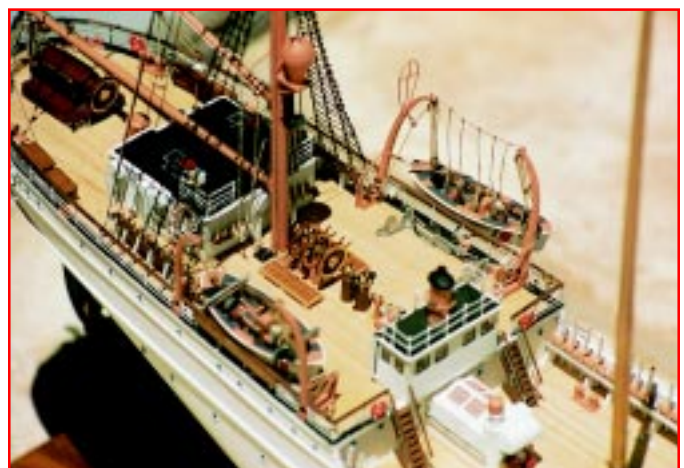
Project: Coast Guard ship model deck details. Wheels, block and tackle and many other small fittings were made easier through the use of miniature machine tools.
