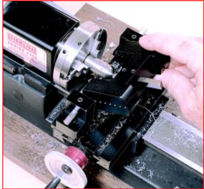
Figure 34 —The radius cutting attachment can cut a convex or concave radius. Unlike most lathe operations, the tool is moved up and down rather than horizontally.
