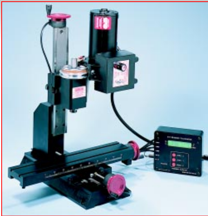
FIGURE 68 —A Sherline mill or lathe fitted with a digital readout makes keeping track of cut and feed calculations much easier. It reads out to .0005" (.01mm) and also provides a continuous spindle RPM display.
