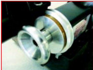
FIGURE 17 —The steel spindle handwheel makes it easier to control the spindle by hand.
