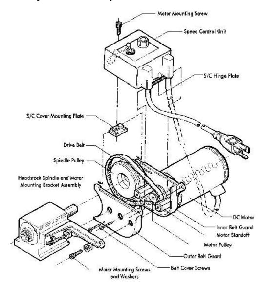
The drawing below shows the components in the 3306 unit and how it is assembled.
