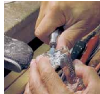
Wagner Dental Lab of Danbury, CT uses CeramCut Blue Stones for grinding chrome cobalt on flexible partial.
