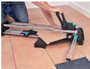
special guide for diagonal cutting
