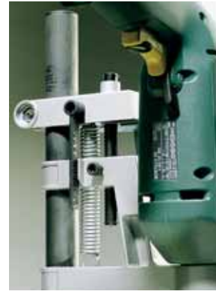
depth of cut set by depth stop
