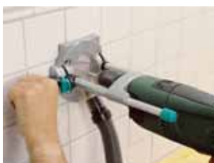
additional handle for precise placement and against skidding when drilling
