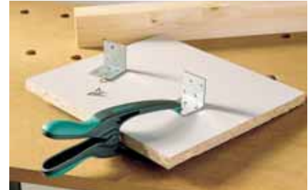
large depth offered by the long clamp arms allows fixing in areas far away from the edge of the workpiece
