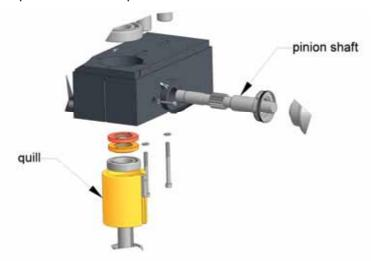
It is not necessary to lubricate the **drilling spindle**, as the ball bearings are fully enclosed and had been lubricated during production for the entire service life of the machine.
