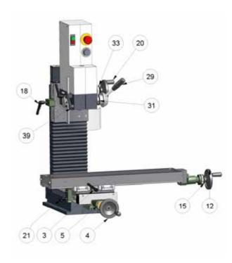
Another possibility of operating the tool spindle is by turning the operating lever (part no. 29). After loosening the clamping lever (part-no. 39) the control lever can be turned. One graduation mark on the collar (part-no. 31) corresponds to 1 mm of travel.
