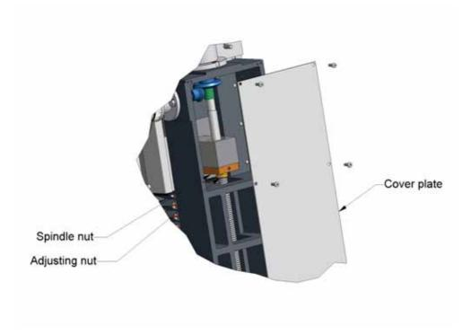
In the case of spindle nuts with ball screw an adjustment is not necessary and also not possible.
